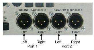
The audio ports do not need to be connected in order to transfer files from the AMR-100I to your computer playback system.
